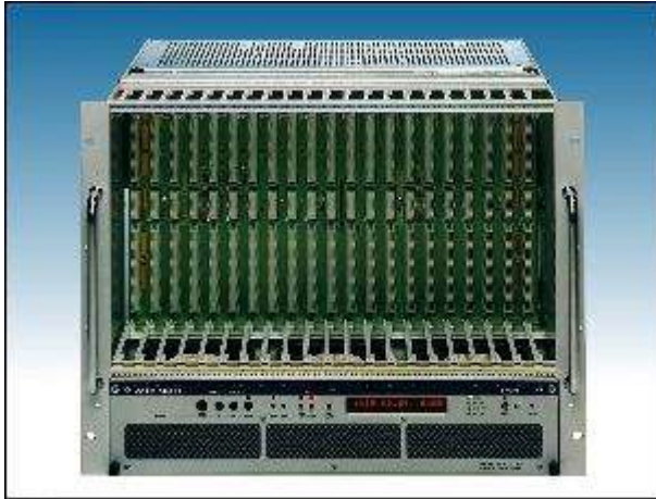
21 slot 6U crate for 19" racks
